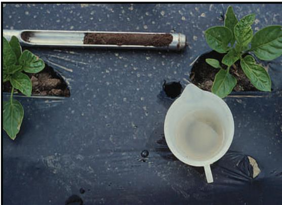
**Figure 4.** Add a small amount of water to the bottom of hole for good contact of ceramic cup to soil.
